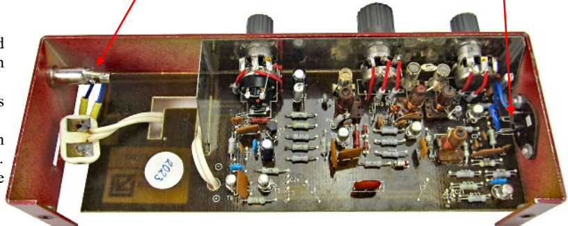
Internal view of a probably later produced Delfin with a jack headphones socket and a fiberglass circuit board.
