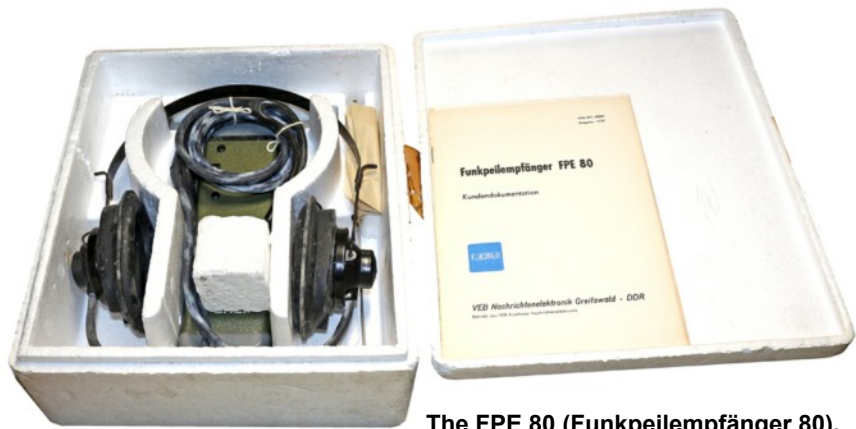
The FPE 80 (Funkpeilempfänger 80), with user manual, headphones, and sense aerial was packed in a Styrofoam box.
